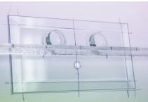
Remove excess glue from the front disc and illuminate the glued discs again for 3-4 minutes.
