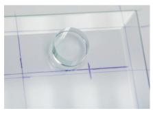
Illuminate the glue with the UV lamp for about 30 -60 seconds. Then remove the excess glue. Now you can glue the front disc.
